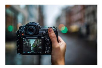
Live View shooting mode is essentially what it says on the tin — you're seeing what the camera's lens is seeing, and what the sensor is recording, but on the LCD rather than through the optical viewfinder.
